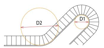
Minimum pulley diameter is also determined by the base belt
